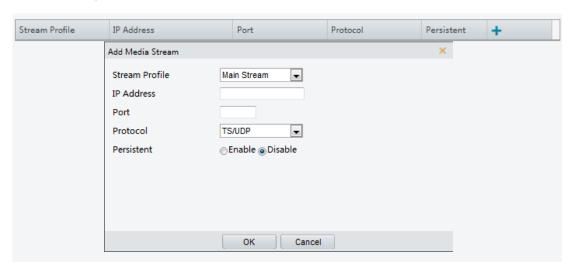
2. Click , select a stream type, and then set the IP address and port number of the unicast or multicast group for the decoding device that receives audio and video streams from the camera.
